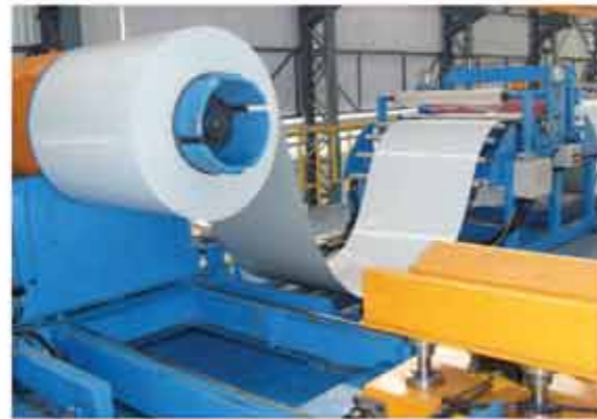
Uncoiler & Coil car
